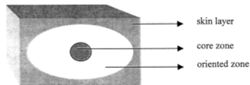
Figure 4 Core, oriented zone, and skin layer illustrated in the cross-section areas of the samples.
